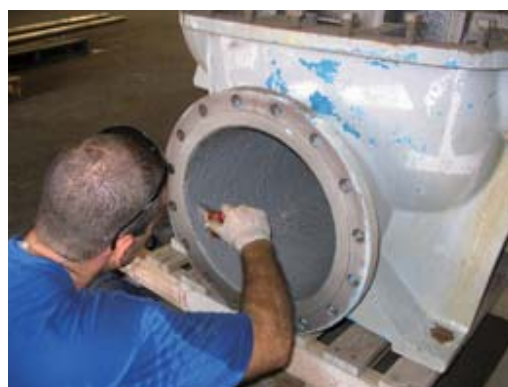
Corr-Paint™ CP2060 coats pump housing.
